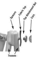
\*5. Unscrew top attachment nut from bolt. Place grommeted fabric top over the bolt, screw on top attachment nut and tighten until snug. Top should rotate easily - do not overtiahten. Repeat this procedure on the remaining arommets.
